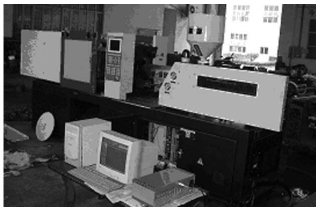
Figure 1 HD-980 hydraulic, dynamic injection-molding machine.
